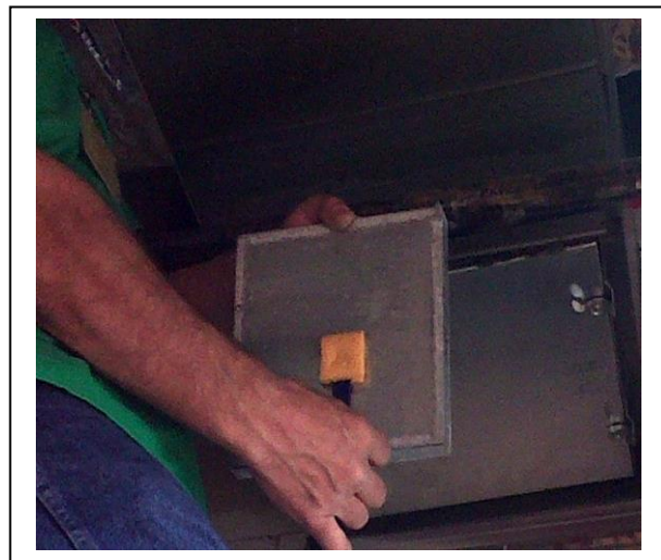
Figure 2. Swabbing bare access panel with Sponge Stick
